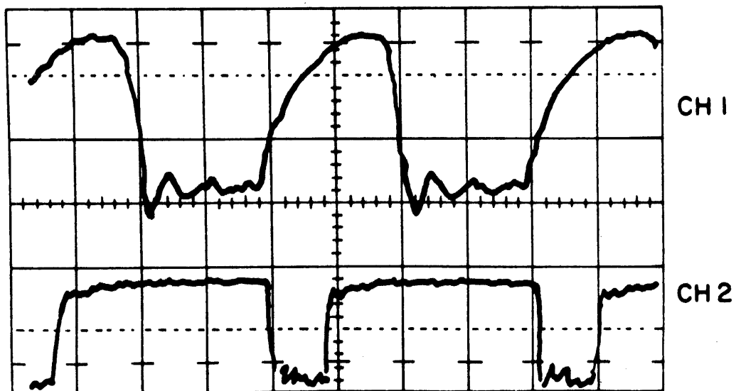
Figure 3-33 Write Driver Output Waveform
